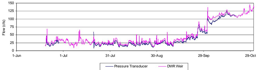
**Figure 2-8 Comparison of flow measured with the permanent station and the temporary pressure transducer at DWR Weir from June to October 2001**
