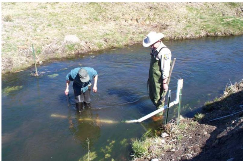
Figure 2-6 Pressure transducer deployment for the cable unit style
