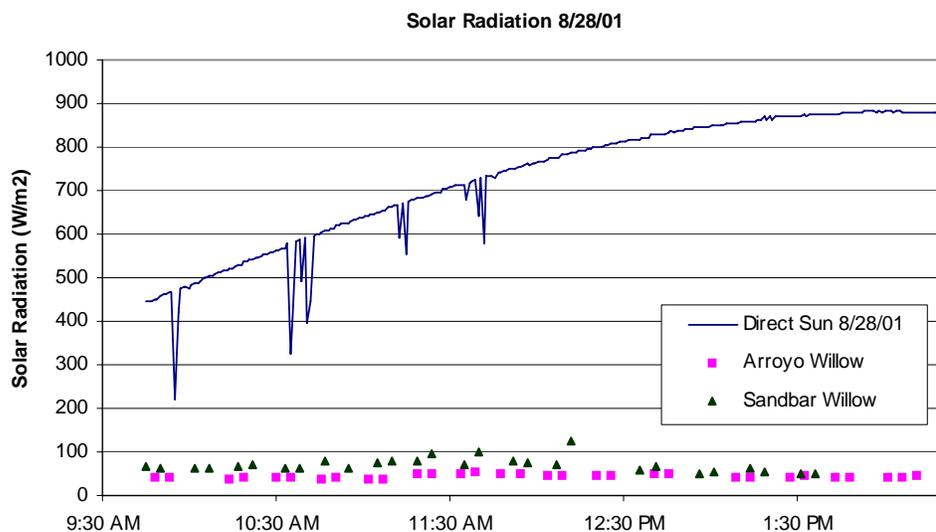
**Figure 2-5 Sample transmittance data**
