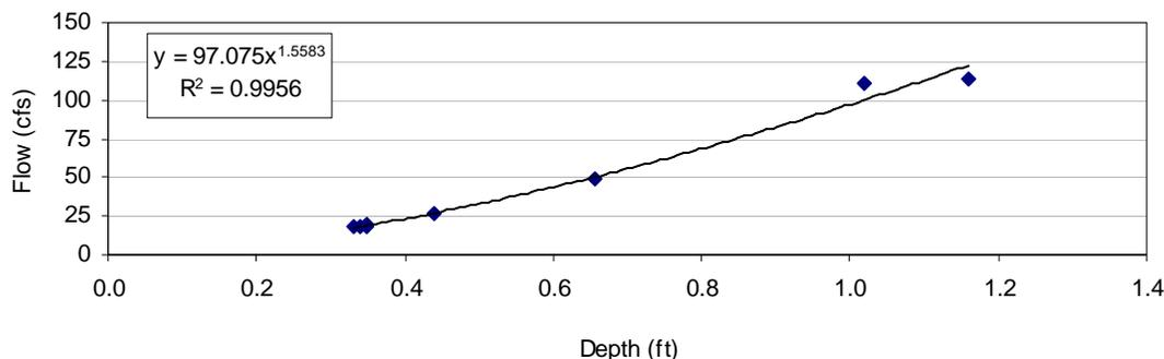
**Figure 2-7 Sample pressure transducer rating curve for Anderson Grade (2001)**
