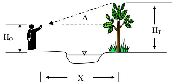
Figure 2-2 Diagram depicting the variables for calculating  $H_T$ , the height of a tree using a Brunton compass
