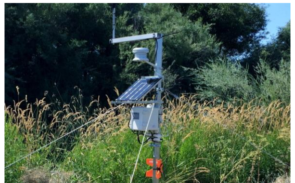
Four new weather stations installed in 2017 with the CA North Coast Water Quality Control Board, for improved monitoring capabilities.
